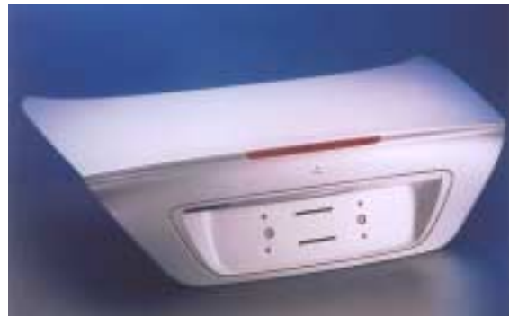
Class A decklid made of SMC (Daimler-Chrysler)
