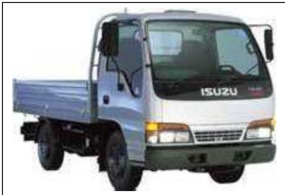
Isuzu Truck uses low density SMC panels
